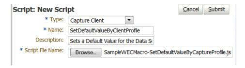
After saving the script, the next step is to assign it to a client profile. In the Capture tab, open an existing client profile, or create a new one. The Profile Type can be either "2 - Capture and Index" or "3 – Index Only". On the Extension Profiles train stop, add the script you just created.
